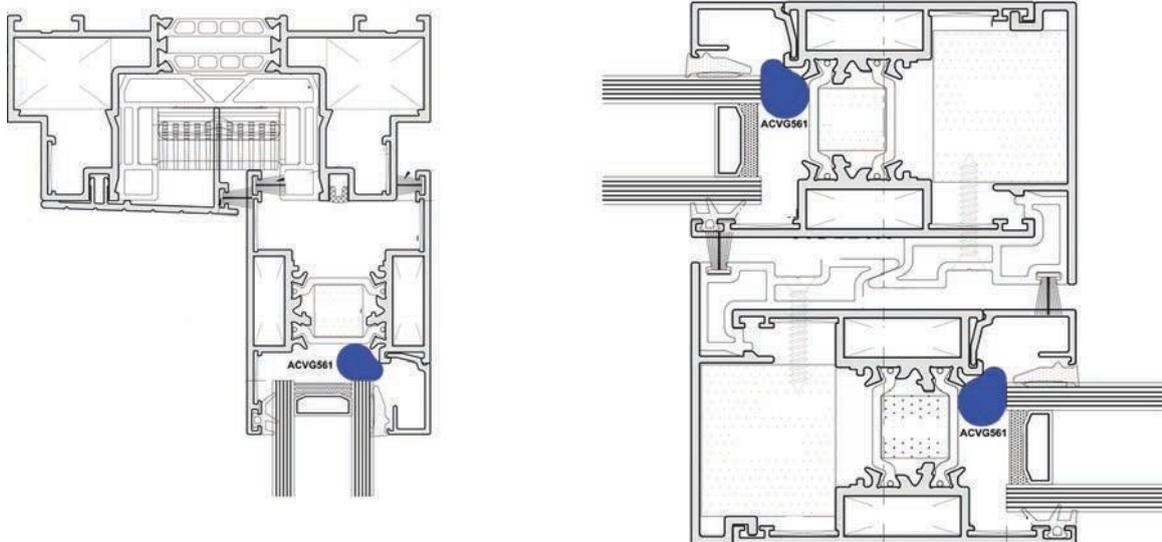
Before starting to glaze please be aware that the glass will be a snug fit. It is designed to be this way to support the interlock and help with rigidity. Also note that the glass should be un-taped.
