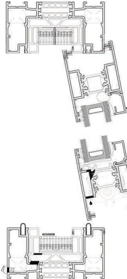
Locate the top of the door sash to the head of the outer frame ensuring the cut-outs line up with the frame.
