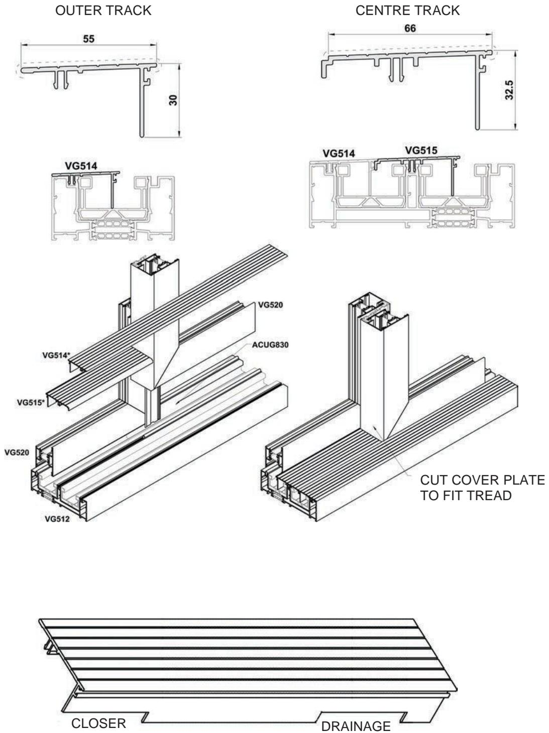
The bottom tread will have notches for the drainage. The notches fit around the frame closers (see FRAME CLOSERS page)
