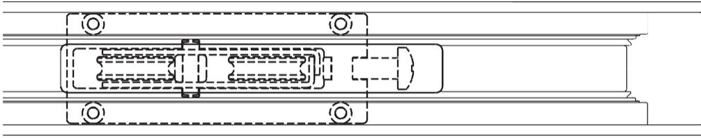
The wheels are supplied in a pre-set position; however, they are not 100% accurate due to tolerance, fitting etc. It is easier to adjust the wheels prior to any glazing or fitting of any guides and trims as they will require removing to gain access.
